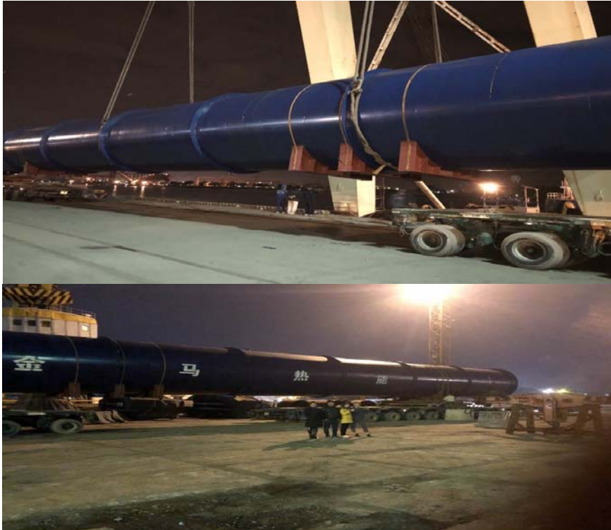
Handling Steam boiler : L38m x Dia 4,0m
